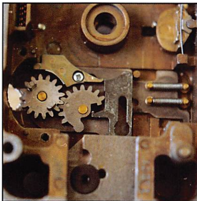
Photo 5: This is the view from the backside of the rack and gear in the normal locked position.
