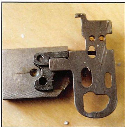
Photo 4: This is how the rack and slide should look when the lock is open.
